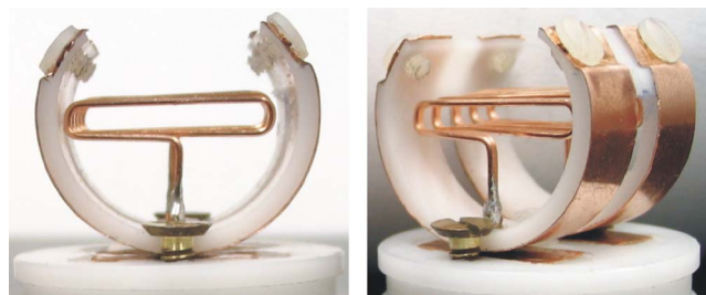
FIG. 3. (Color online) Photographs of a rotatable flat coil holder built for a Chemmagnetics Apex DRNS Wideline static solid-state NMR probe.
